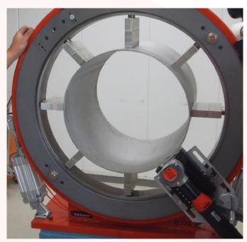
The precision of our cutting machine allow a perfect tube to tube alignement, with the smallest gap possible, removing the need to facing the tube therefore saving a significant amount of time and money.
