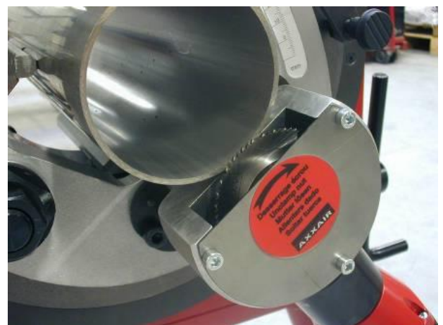
Exterior tool installation
