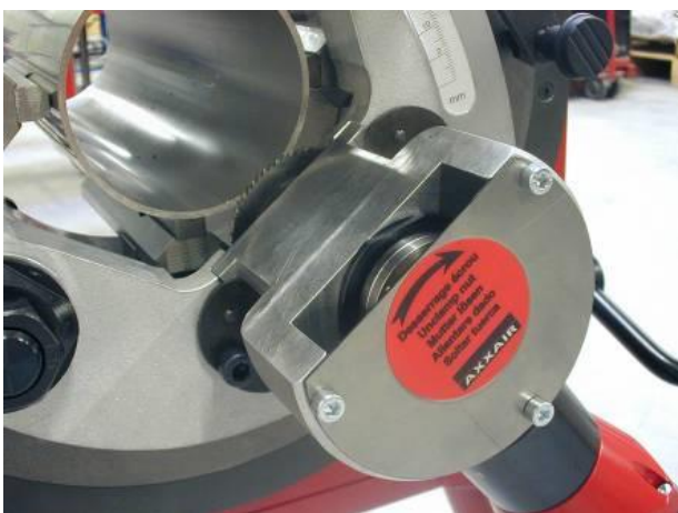
Tool installation near the jaws
